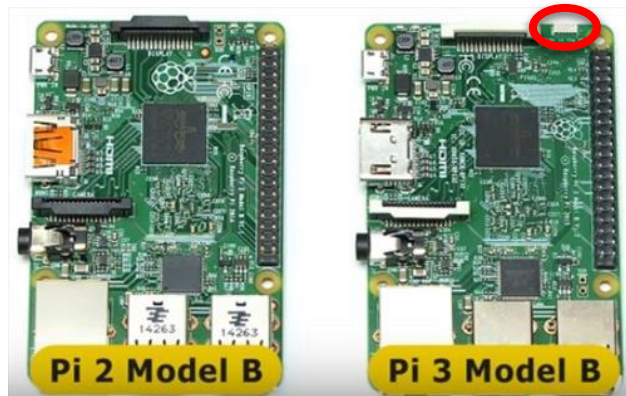
Figura 13: Antena Wi-Fi incluida en Raspberry Pi 3. [9]
