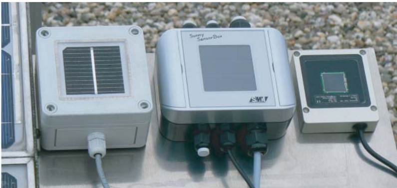
Figure 9.3 Various reference sensors of c-Si solar cells at the experimental rig of the Münster University of Applied Sciences: The modules are installed at module level to measure the incident radiation on the solar module.
