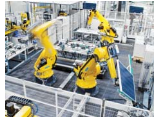
Installation of the module frames
