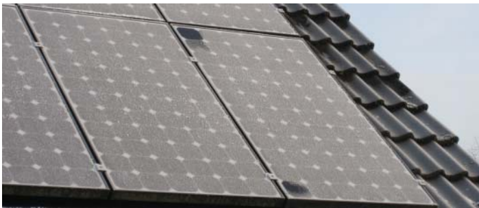
Figure 9.12 “Thermography for the poor” on a cold November day: The two cells of the modules from Figure 9.10 can clearly be seen as free from hoarfrost. Photo: T. Stegemann, Münster UAS.
