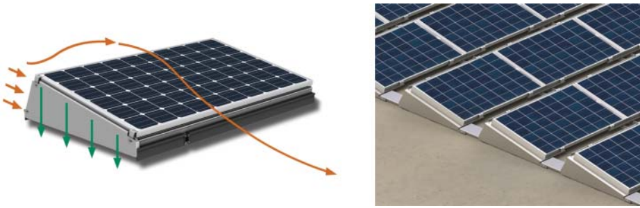
Figure 6.32 Solution for roofs with low bearing capacity: Because of the low closed form, the system offers hardly any resistance to the wind; instead, the elements are pressed down by the wind. Source: LORENZ-Montagesysteme GmbH.
