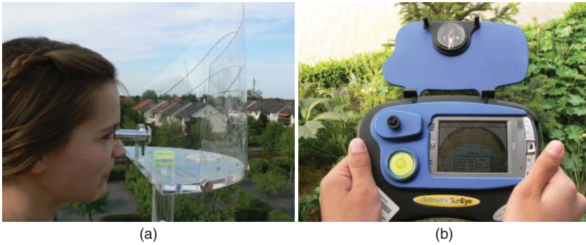
Figure 10.2 Two variants of the shading analysis: The panel (a) shows the manually operated Sun path indicator and the panel (b) shows the SunEye device that permits automatic acquisition of the shading horizon.
