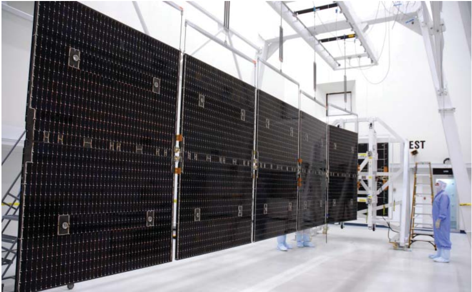
Figure 1.14 Modern solar array of the space probe Dawn with a power of 5 kW. Source: NASA.
