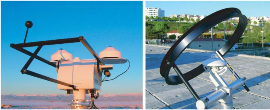
Figure 9.5 Sensors for measuring diffuse radiation: Whereas the shade ball variant must continuously track the Sun, the shade ring is satisfied with an occasional adjustment of the tilt angle. Photos: Kipp and Zonen.
