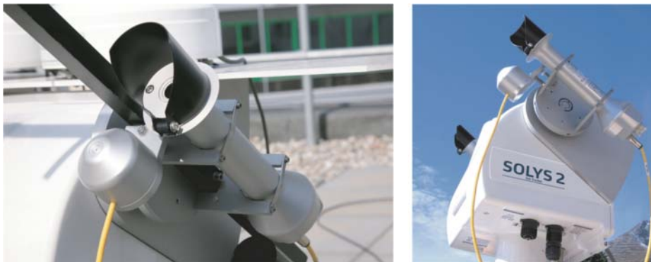
Figure 9.4 Pyrheliometer for measuring direct radiation: The instrument must continuously track the Sun. Photos: Kipp and Zonen.
